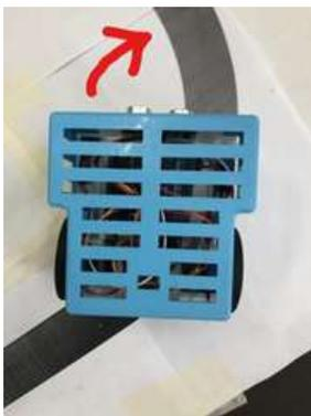
The left sensor is on the black line and the right sensor is on the white line, the robot must turn to the right..
