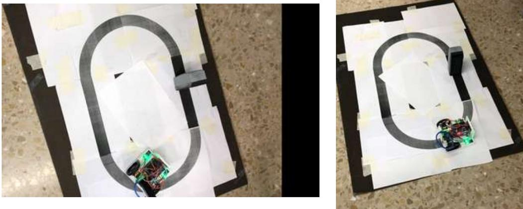
It can be programmed so that it does not leave the circuit, i.e. when it detects the black line, it turns inwards. Another option is to make a sumo, with glasses inside the circuit and it must lead out of the circuit.
