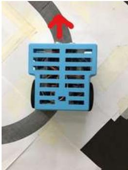
The two sensors do not detect the black line, so it must move in a straight line.
